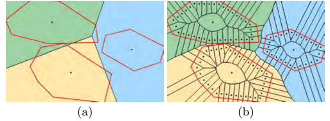
Figure 7: Comparison of assemblage methods. The red polygons are I-Regions . (a) A straightforward Voronoi segmentation. Notice some I-Regions are eroded in this example. (b) Our approximated region-based Voronoi approach.
