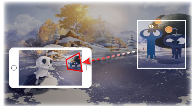
Figure 1. Outside-In is a visualization technique that re-introduces off-screen ROIs onto the main screen as spatial PIP previews, allowing users to make sense of where off-screen ROIs are.
