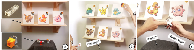
Figure 3. Display rack in a smart showroom. (a) An RFIMatch module is mounted behind each item. Several RFIMatch fingerstalls are provided with voice guidance in different languages. (b) A visitor wearing the German fingerstall hears the embedded audio message in German by touching the icon. (c) Two users wearing different fingerstalls greet each other in their own languages.
