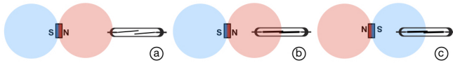
Figure 5. Operating principle of a reed switch. A reed switch is (a) normally open, but (b) closed by an external magnetic field, regardless of (c) polarity.
