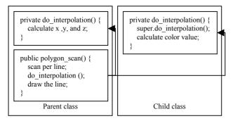
Figure 3 The example of using function overriding.
