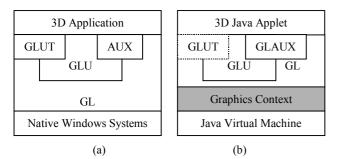
Figure 1 The hierarchy of (a) OpenGL and (b) JavaGL modules.
