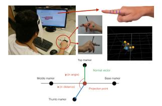
**Figure 4:** Experiment apparatus (left), including markers (middle) and Vicon tracking system (right). Upper right: instruction in the experiment shown on the monitor. The red point means the target. Down: the thumb position computed in SegTouch.
