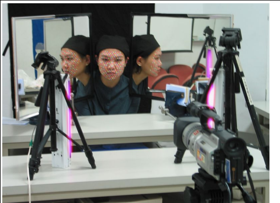
Fig.2. The tracking equipment. This photo is taken under normal light. Two “Blacklight Blue”(BLB) lamps are placed in front of a subject and mirrors. The low-cost special lamps are coated with fluorescent powders, and it can emit long wave UV-A radiation to excite luminescence.
