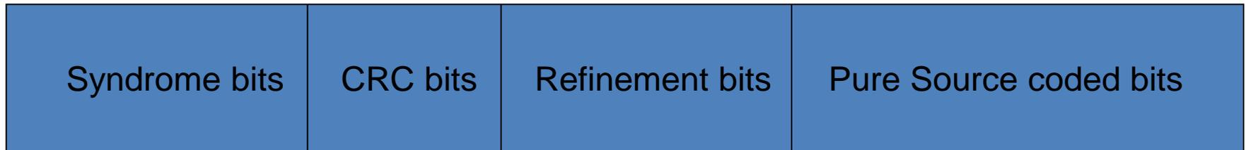
Bit stream syntax associated with a block.
