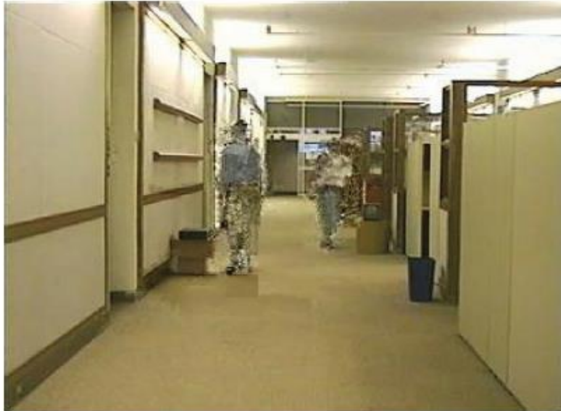
Fig. 2. Privacy preserving encryption: DCT coefficients permutation (figure taken from [13, Fig. 2(b), p. 1171]).
