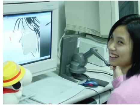
Figure 1: System configuration. A PHANTOM force feedback device is provided for users to draw the Chinese painting with haptic perception.
