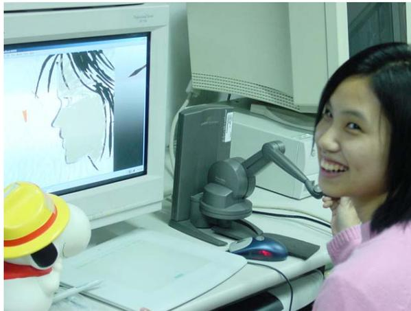
**Figure 1: System configuration. A PHANTOM force feedback device is provided for users to draw the Chinese painting or calligraphy with haptic perception.**
