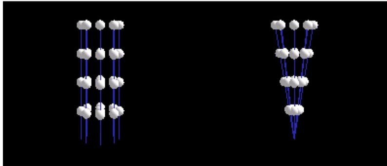
Figure 3: The 3D bristles models, model A and model B, where the hair should be vertically but in actual use, the water condensing force keeps all hair in a cone shape.
