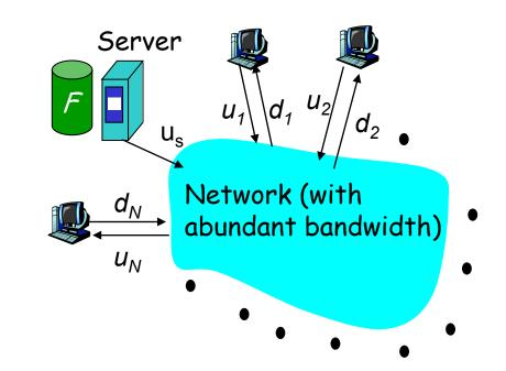
Time to distribute F to N clients using =  $d_{cs}$  =  $\max \{ NF/u_s, F/\min(d_i) \}$  client/server approach
