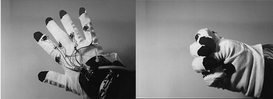
**Photo 1.** *Sensing Glove with five tact switches.*
