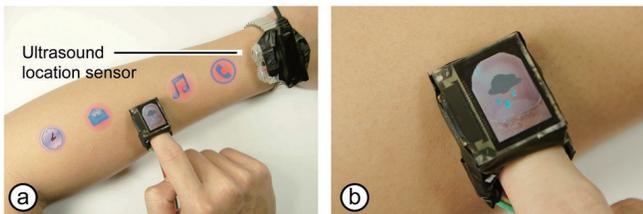
**Figure 6.** Positioning of invisible virtual buttons in line along the arm. (a) Users acquires the latest weather conditions by tapping on where the icon is located on their arm. (b) Close up view of *NailDisplay*.
