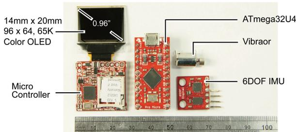
**Figure 2.** *NailDisplay* prototype, which consists of a 0.96" OLED display module, ATmega32U4 microprocessor, and sensors such as a 6DOF IMU and a vibrator, depending on the experimental applications
