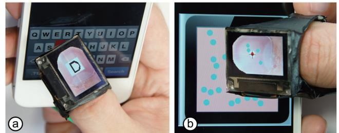
**Figure 4.** (a) Use of *NailDisplay* to type on a virtual keyboard by revealing the key of press. (b) The occluded content shifts to *NailDisplay*, allowing users to point to a small target. Notably, in this application, a watch size screen is simulated on a large touch screen.
