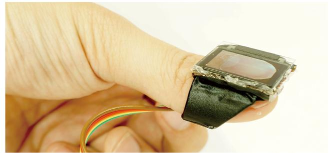
**Figure 3.** Resulting screen on the fingernail, which is 5mm-thick. The prototype is combined with an adjustable finger ring, allowing for easy use. The portion around the fingertip is left open for native haptics.
