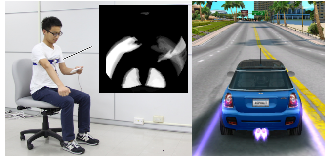
Figure 1. Cyclops is a wearable single-piece bodily gesture input device that captures an ego-centric view of the user. With Cyclops worn at the center of the body, the user plays a racing game on the mobile phone with hand and foot interactions. The user pushes forward an imaginary gear stick on his right to trigger a nitro turbo.
