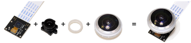
Figure 4. Cyclops’ ultra-fisheye field-of-view is realized by firstly replacing the lens in the NOIR camera module with a 110-degree lens, and then bridging it with a 235-degree super fisheye lens.
