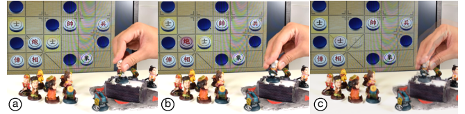
Figure 7. Chinese chess allows for moving multiple chess in the same-class chess (e.g. two guards) at the same time. A user makes a move by (a) placing a character on the commander platform, (b) rotating it to target direction, and (c) stamping it to defeat the enemies.
