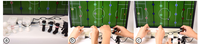
Figure 11. Table Football allows remote users to play together. (a) Four tagged handles and two stages with a slider cap are provided to each team. The players (b) play the game by placing the desired handles on the stage, and then they try to take possession of the ball by moving the handle along the slider. (c) Once possession is gained, the player sets the target direction by turning the handle, and kicks the ball by stamping the handle on the stage.
