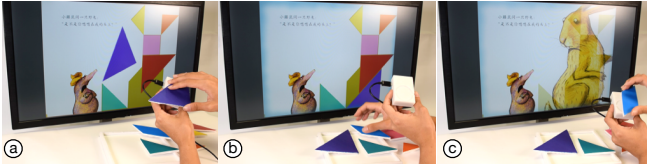
Figure 6. Tangram Reader allows the reader to read the story book by assembling Tangram pieces. The reader can assemble the pieces of the tangram by (a) placing, moving and rotating a piece into the desired position. (b) When a player becomes stuck, the system provides a color as a hint. (c) When the shape has been completed, the hidden character appears and the story continues.
