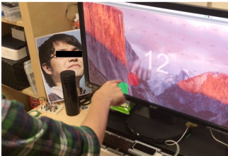
Figure 3: Task of user study 2: users are asked to push buttons randomly assigned on 27-inch screen with their index finger which is sensed by Leap Motion with and without Shadow system.
