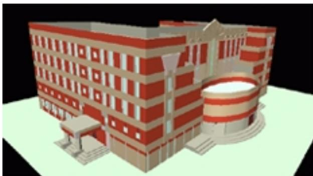
Figure 9 This building model contains 5,273 polygons with 12 kinds of materials with VRML format.
