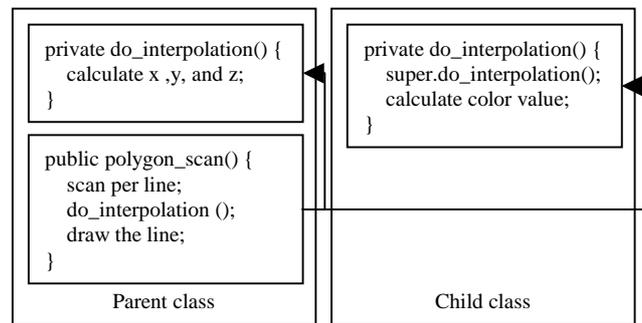
Figure 3 The example of using function overriding.
