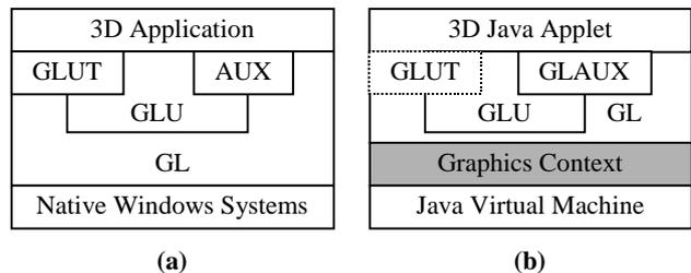
Figure 1 The hierarchy of (a) OpenGL and (b) jGL modules.
