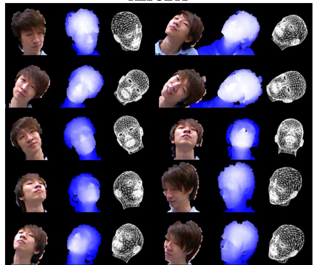
The results of a user who makes ten arbitrary pose. The first and fourth columns show what pose users make. Note that our system doesn't take any advantage from these color images so that it still performs well when there is no lighting in the environment.
