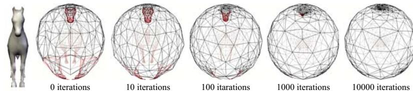
**Figure 3:** Embedding a polyhedral object on a sphere using relaxation. Initially, the vertices are projected through an interior point of the model onto a unit sphere. The relaxation is finished when all faces are oriented correctly. Incorrectly oriented faces are surrounded by red edges.
