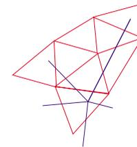
Figure 9: Edge-edge intersections are determined by following an edge (blue in this illustration) over the faces of the other triangulation (red). After finding an intersection the face-to-face coherence exploited and only the edges of the next face are tested.
