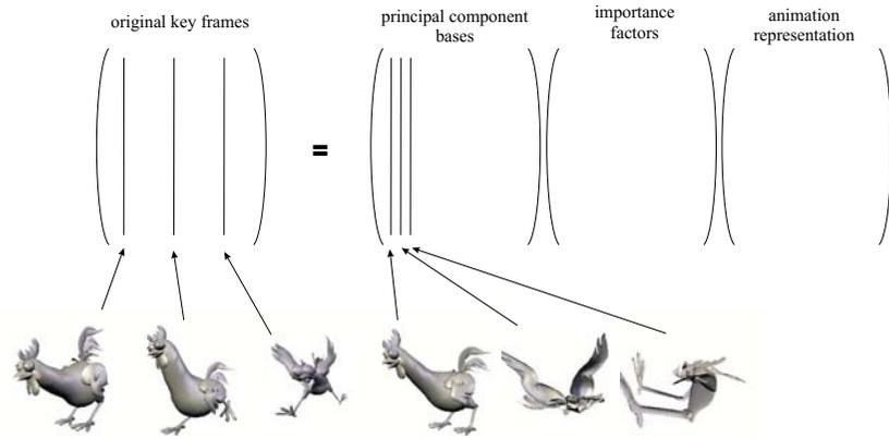
**Figure 21:** The SVD applied to a space of meshes. Here the original space represents a key frame animation, the result allows to represent the same animation with less geometries containing most of the original animation's energy.
