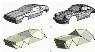
**Figure 6:** In the approach of Kanai et al.<sup>35</sup> the user selects only corresponding vertices and which have to be connected. The mesh is the dissectioned using shortest path connecting the vertices. Reprinted from Kanai et al.<sup>35</sup>.
