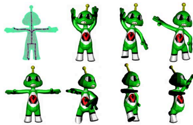
Fig. 8. A transferred skeleton-driven animation generated by our system. The skeleton is nicely shaped according to the character model (upper-left) and the motion can also be transferred from the fat man model shown in Fig. 1 (left).
