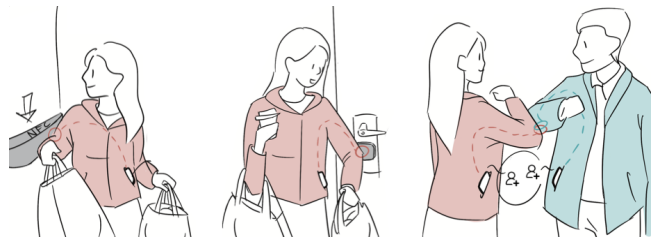
Figure 1: Body-centric interaction with NFC devices through a piece of near-field enabled clothing, which extends the reading range of a mobile device's NFC to the user's protruding body landmarks (e.g., elbows) for touch interaction.
