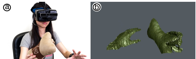
Figure 2: (a) A RealSense camera is used to capture the depth image and (b) duplicate it in the virtual space.
