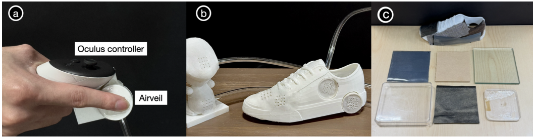
Fig. 14. Airveil demonstration setups. (a) Airveil mounted on a VR controller using a support frame; (b) Physical 3D models (a shoe and a humanoid figure) integrated with Airveil; (c) The reference set of physical material props used to establish ground-truth tactile expectations.
