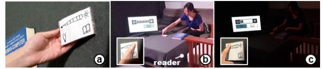
Figure 25. (a) Self-made control panel; (b) and (c) dimming the light.
