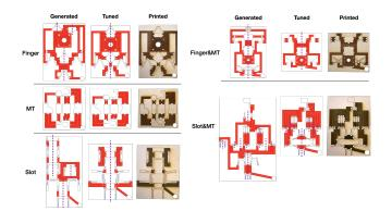
Figure 9: *Daedalus*-generated SVGs (left), tuned SVGs by an occupational designer (center) and printed laser-cut plates with assembly components removed (right). Dotted lines indicate layer-local and within-component lines of symmetry in the *Daedalus*-generated layouts, and global lines of symmetry in the tuned layouts. (Note: the MT layout and the top of the SlotMT layout do not have lines of symmetry, because these model parts are inherently asymmetrical.)
