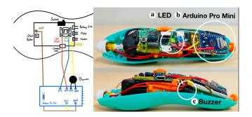
Figure 9: Circuit connection and a modified 3D printing pen. Left: Simple circuit connection between an Arduino Pro Mini (Fig. right b), a buzzer (Fig. right c), and an LED light (Fig. right a) on the 3D printing pen. Right: Displays a dismantled and modified 3D printing pen.
